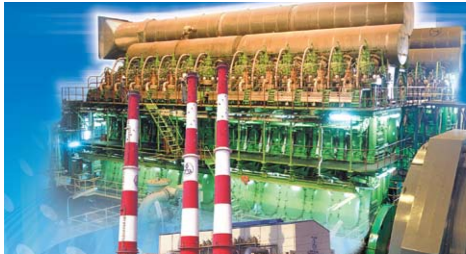
GMR Vasavi 200MW Diesel Power Plant, India(HYUNDAI-MAN B&W 12K90MC-S x 4)
