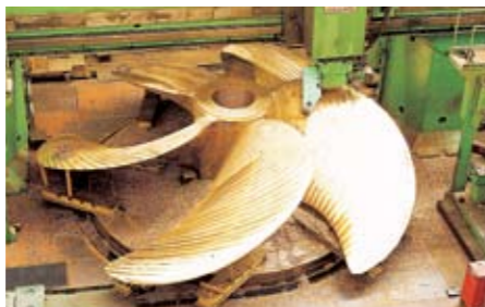
1. World's Largest Propeller Weight 110.2 tons Diameter 10.4 m Blade 5 Shiptype 18,800 TEU Container-ship
